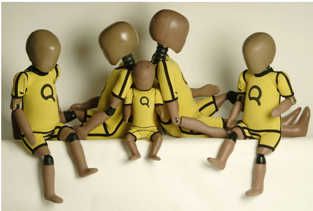
Figure 1: Q-series of child dummies (left to right Q1.5, Q3, Q0, Q6 and Q1)
